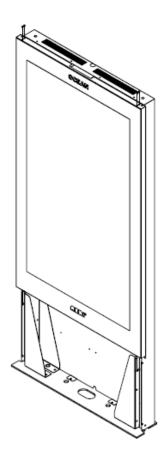
Secure the glass by using 4 screws on the top and 4 screws at the bottom of the glass frame
