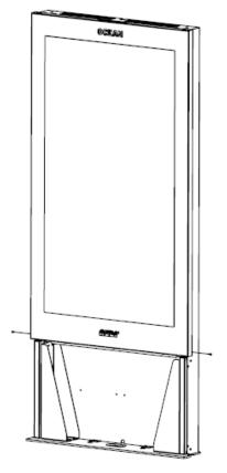
Use the screws on each side to lock the glass frame
