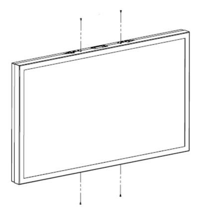
Attach front cover with screws
