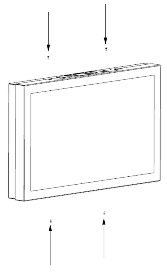
Attach front cover with screws
