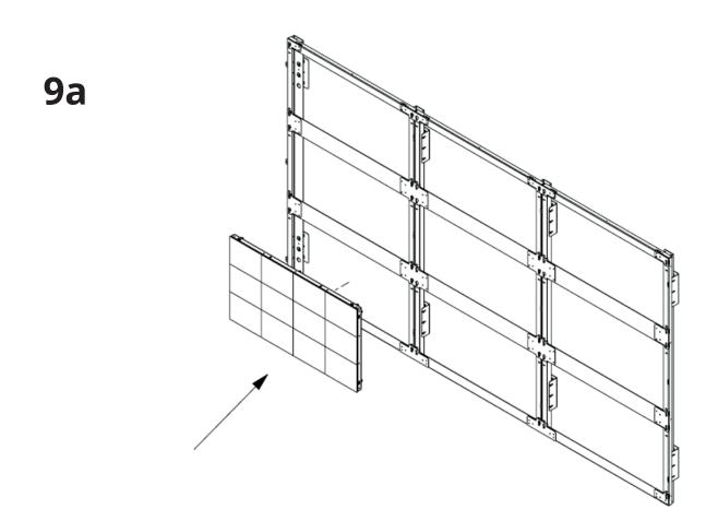
Attach the LED Module. Start with bottom left corner and continue up
