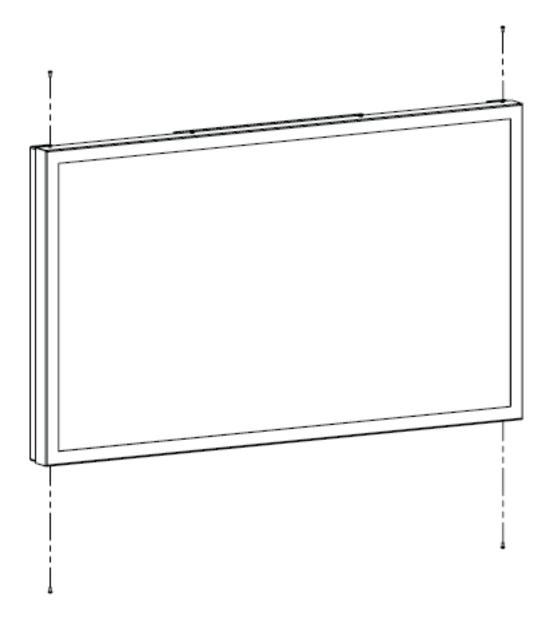
Attach front cover with screws
