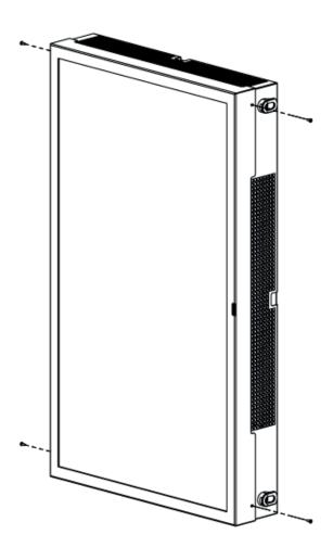
Attach front cover with screws
