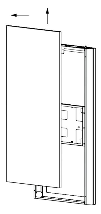
Remove back cover by removing screws
