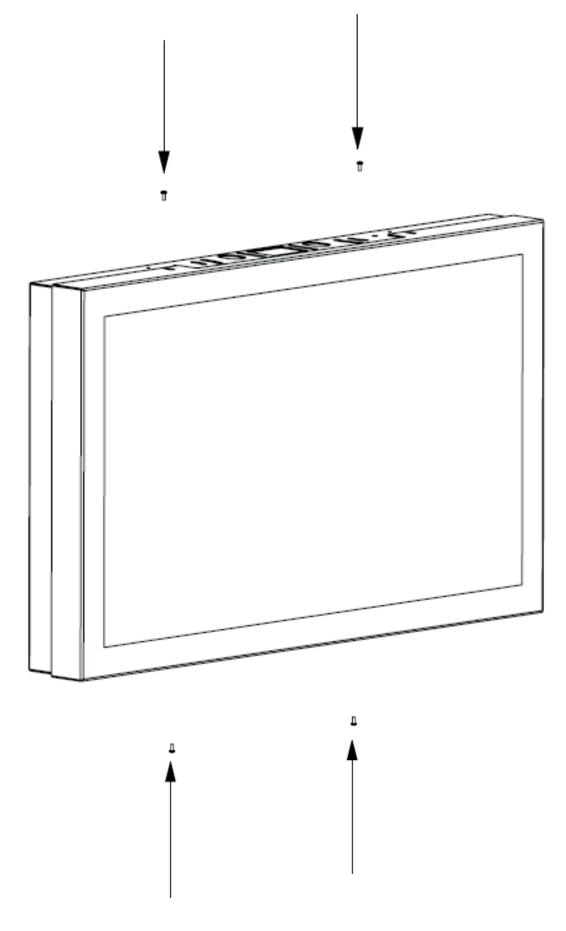
Attach front cover with screws
